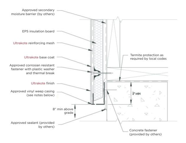
NOTE: Maintain 1/8" space between beveled insulation and weep casing bead.
